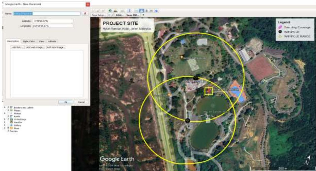
Figure 5. Wi-Fi Poles Coordinate and range placement in Google Earth Pro
