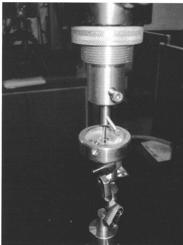
Figure 5: Specimen placed into the custom-made jig for push-out test.
