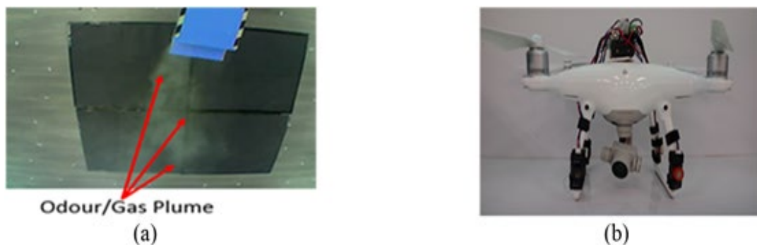
Fig. 24. The experiment setup. (a) Chemical plume generator and (b) Quadrotor armed with four gas sensors.
