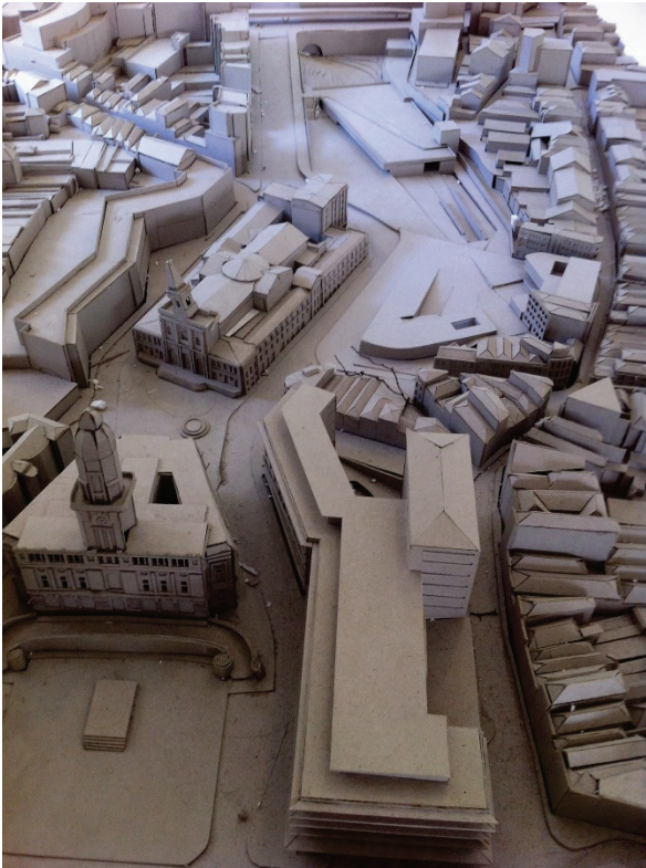
Photo 2: This is a second year design studio 1:500 scaled model which was done with mounting boards so that it can be detailed including the windows and allows the individual model to be slotted in.
